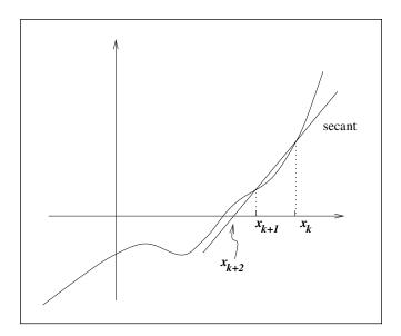
**Figure A.3** One step of the secant method for a scalar equation.
