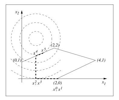
**Figure 16.3** Iterates of the active-set method.
