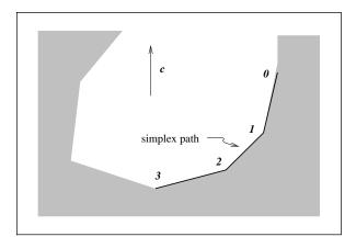
Figure 13.3 Simplex iterates for a two-dimensional problem.
