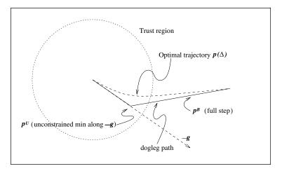
**Figure 4.4** Exact trajectory and dogleg approximation.
